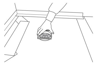
**11)** Cut the top piece (4) to the right length to match the thickness of the tiles, and position in place.
