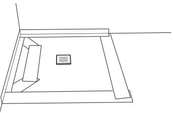
**12)** Position the grate (3) in place. The shower element is ready for tiling.
