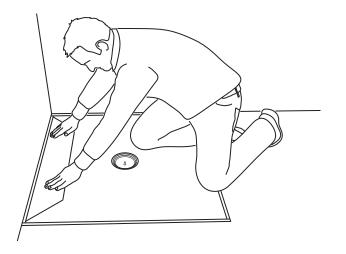
8) Position the pipe duct element (2) in the screed recess and press firmly into place.  $BOARD-FIX^{\otimes}$  (6) special adhesive and sealing agent guarantees the durable seal integrity of the bond.
