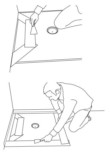
**10)** Before inserting the odour trap, first grease the inside edge of the drain.
