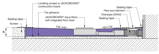
Min. installation height (h) = JACKOBOARD $^{\circ}$  Aqua Reno (65 or 75 mm) + 5 mm tile adhesive
